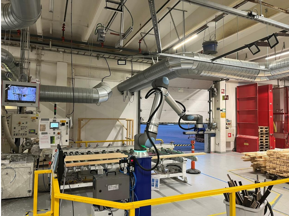
Figure 5.1: Overall system layout showing the UR20 cobot, vision camera, pallet position, and conveyor line.
