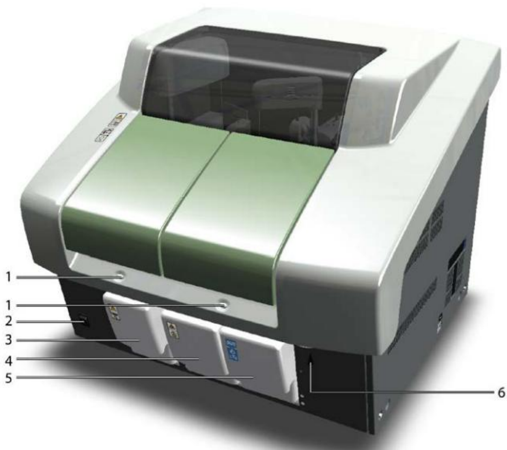
Figure 1. Thermo Scientific™ Gallery™ discrete analyzer exterior with marked positions that correspond to the following 1. operation buttons, 2. main switch, 3. cuvette waste bin, 4. waste container, 5. water container, and 6. lock handle under the main cover [19].
