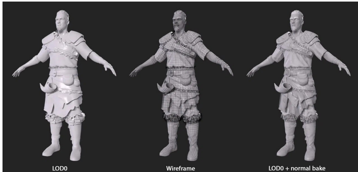
PICTURE 11. A low-poly model, its wireframe and the model with high-poly normal map details (Thunder Cloud Studio 2024a).
