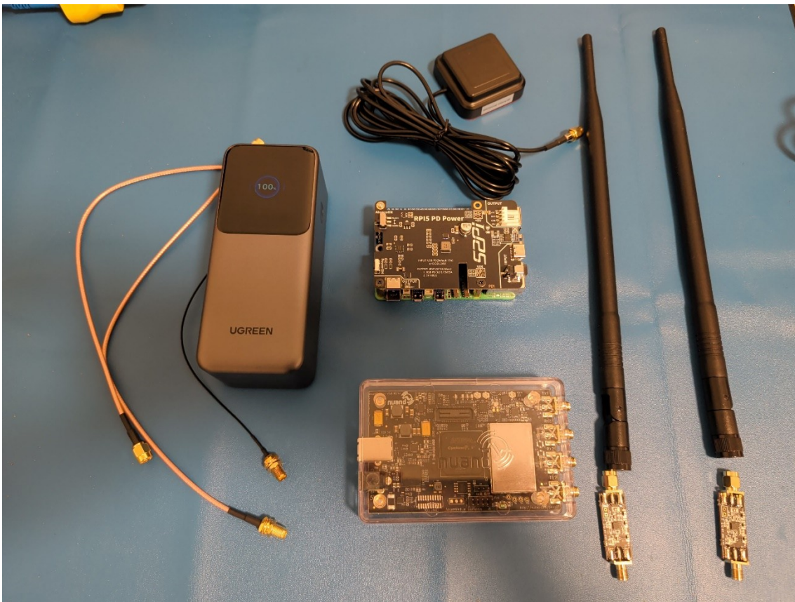
FIGURE 5. Receiver prototype hardware components used in the implementation (laid out before integration).
