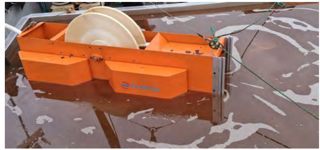
Figure 13. In the ELASTEC X30 Grooved Disc skimmer, the discs are grooved to improve collection capacity by increasing the adhesion area for oil. Photo: Manu Kettunen, 2025.
