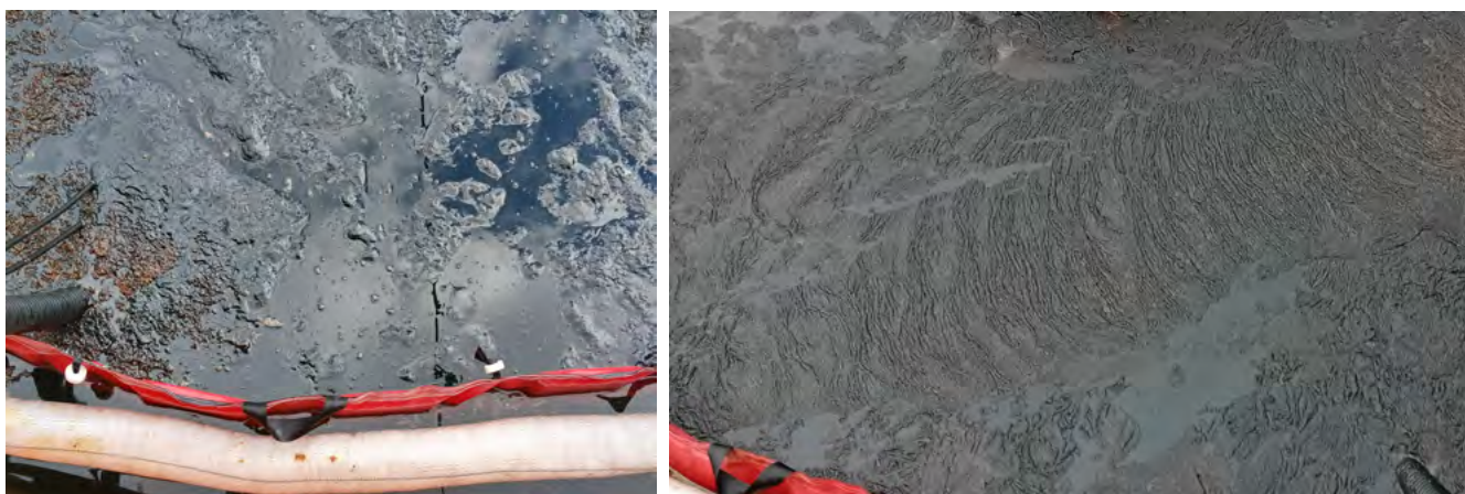
Figure 1. Ultra-low-sulphur marine fuel (RMD80) that has spilled into water begins to solidify at relatively high temperatures, posing challenges for its removal. Photos: Justiina Halonen and Manu Kettunen, 2025.
