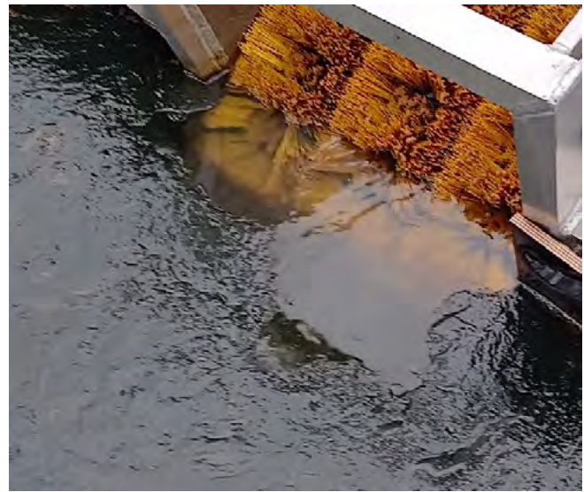
Figure 4. A stationary bow collector forms a water barrier in front of the brushes when rotated upwards. The photo above features MDO DMB marine diesel oil, and the photo below depicts RMD80 fuel. Photos: Justiina Halonen, 2025.
