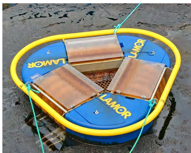
Figure 12. The RMD80 was in a fairly viscous state and adhered well to the brushes once drawn to the device. The oil was recovered, but it was accompanied by a large amount of water. The water temperature was 16°C. Photo: Manu Kettunen, 2025.
