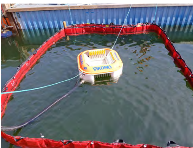
Figure 8. Komara Midi 4 disc skimmer in calm waters at the beginning and end of a skimming operation. The skimmer removed virtually all of the diesel oil without having to change position or assist with the oil supply. Photos: Justiina Halonen, 2025.
