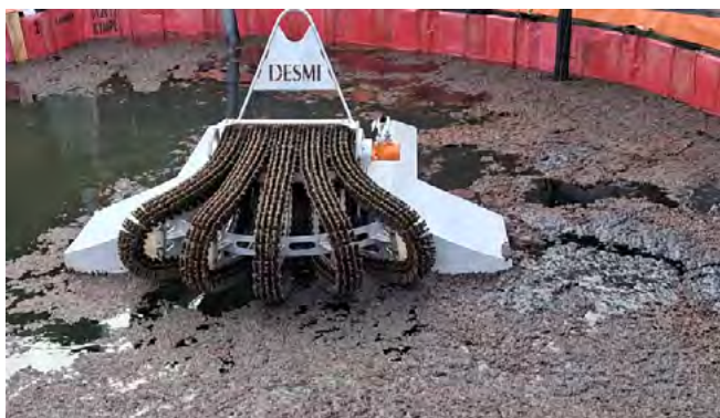
Figure 15. Octopus proved to be an efficient recovery device thanks to its thrusters. The photo clearly illustrates the porridge-like consistency of RMD80 fuel in water at a temperature of 8°C. Photo: Manu Kettunen, 2025.
