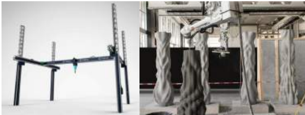
Figure 6: Comparison of Gantry-based (Duran et al., 2019) and Robotic-Arm 3D Printers (Pall, 2023)
