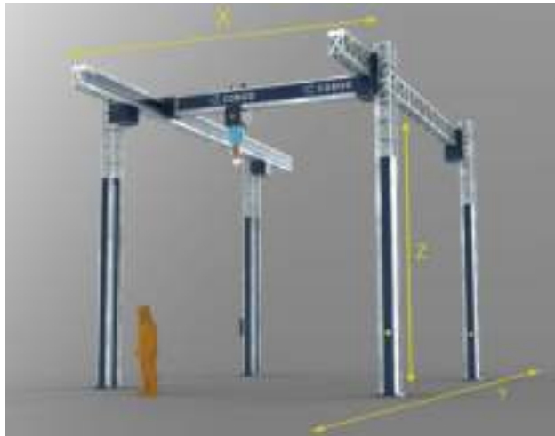
Figure 3: Gantry-based construction 3D printer (industry4blog, 2022)
