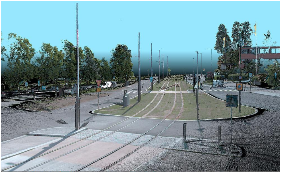
Figure 38. Post-processed Jokeri Light Rail point-cloud obtained by mobile scanning process [77].
