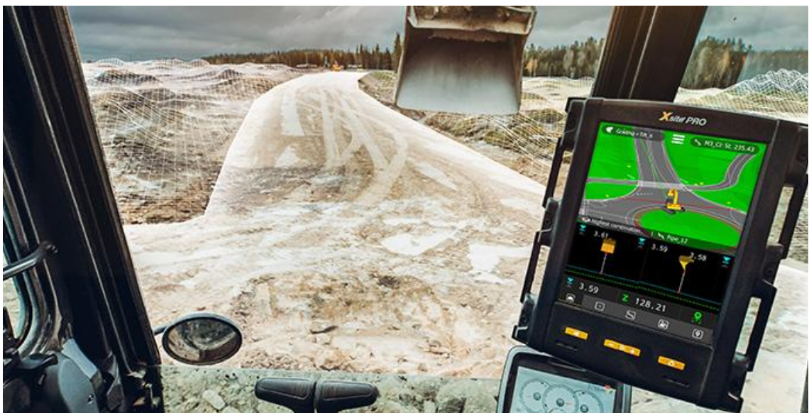
Figure 66. Xsite machine control tablet in use [79].
