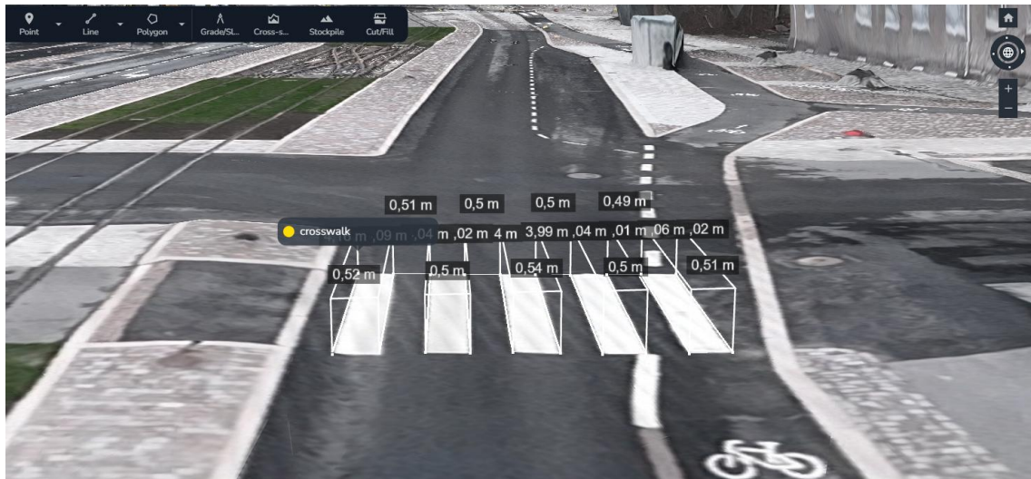
Figure 20. Drone survey-based mapping workflow in Propeller
