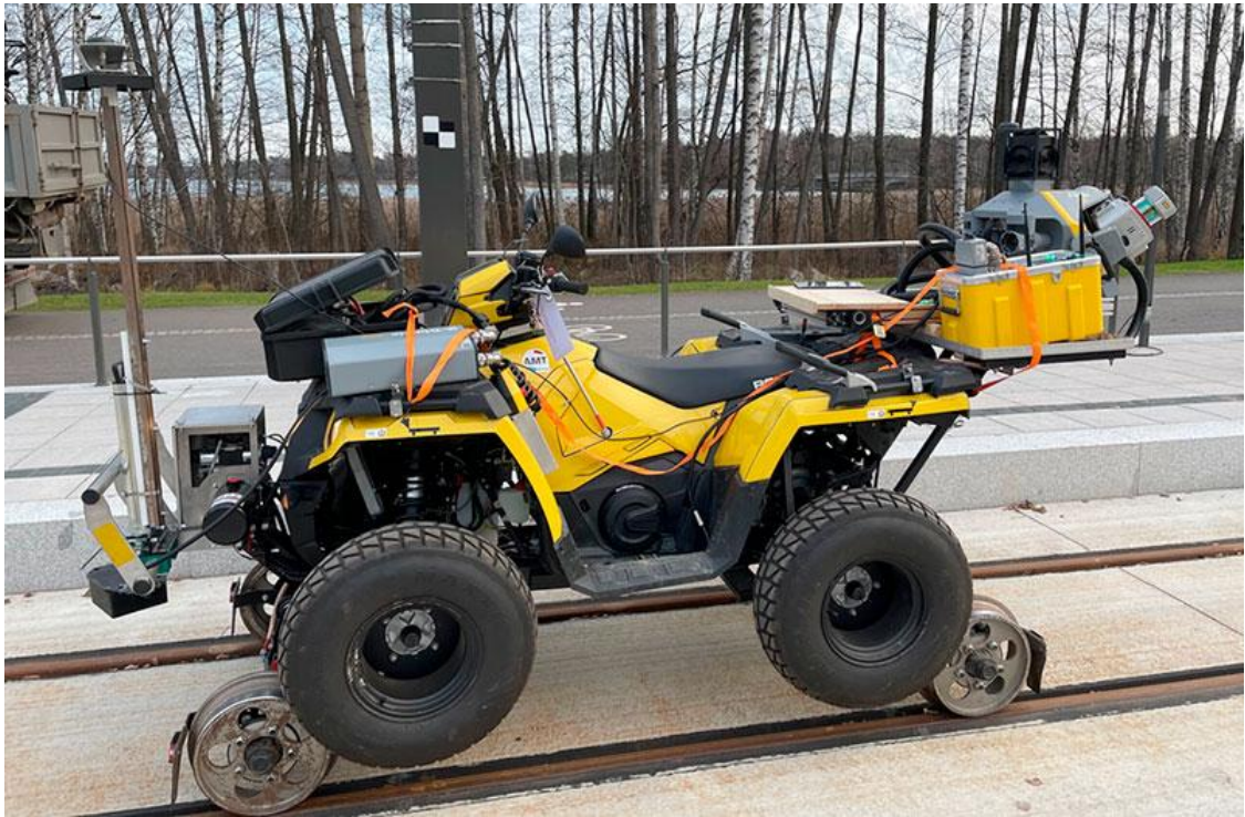
Figure 37. Trimble MX9 Mobile mapping system mounted on a rail quad bike
