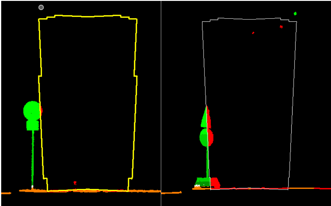
Figure 39. Permanent and temporary traffic signs intruding into the clearance envelope space [75].
