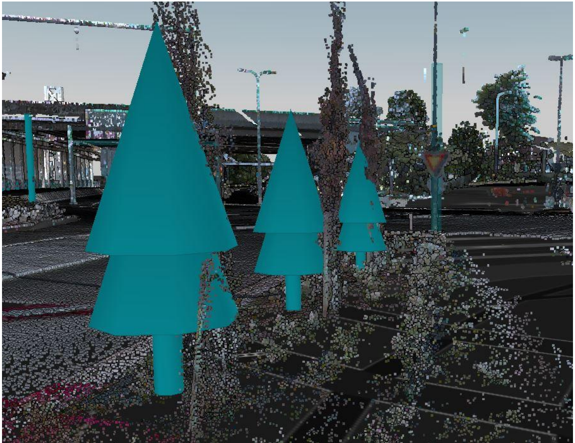
Figure 80. The point cloud and the BIM model comparison
