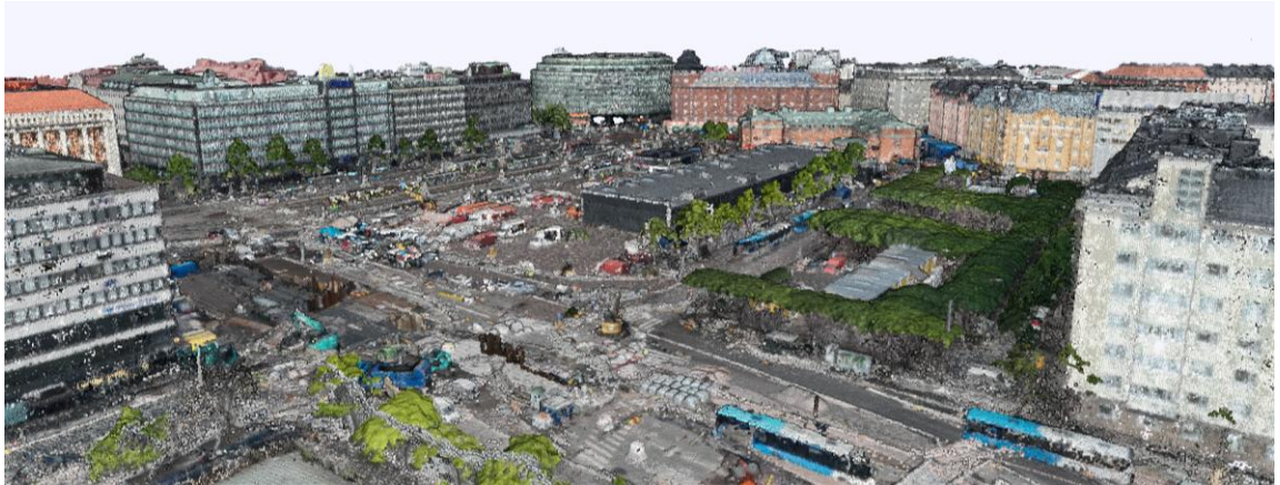
Figure 19. Point cloud obtained from a drone survey
