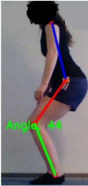
Figure 17 An illustration of a CV-based markerless HPE application (OpenPose) measuring the knee joint. The figure is reproduced from Hellsten et al. (2021) from Rehabilitation Process and Outcome under the Creative Commons Attribution 4.0 International license (Study III).
