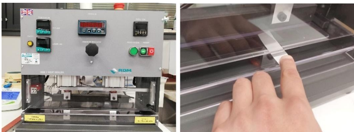
Fig. 6. RDM heat-sealer (left) and heat-sealing of a sample (right)
