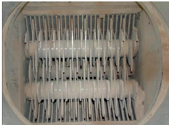
Figure 3.11 The internal structure of a four shaft bag breaker (oharacorp,2015.)
