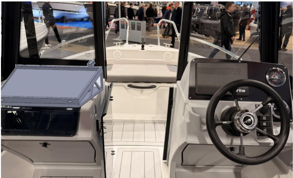
Figure 23. The nautical chart stand on a Terhi 480, here for the co-operator of the vessel to use (Wilhelm Guarnieri, 2026)
