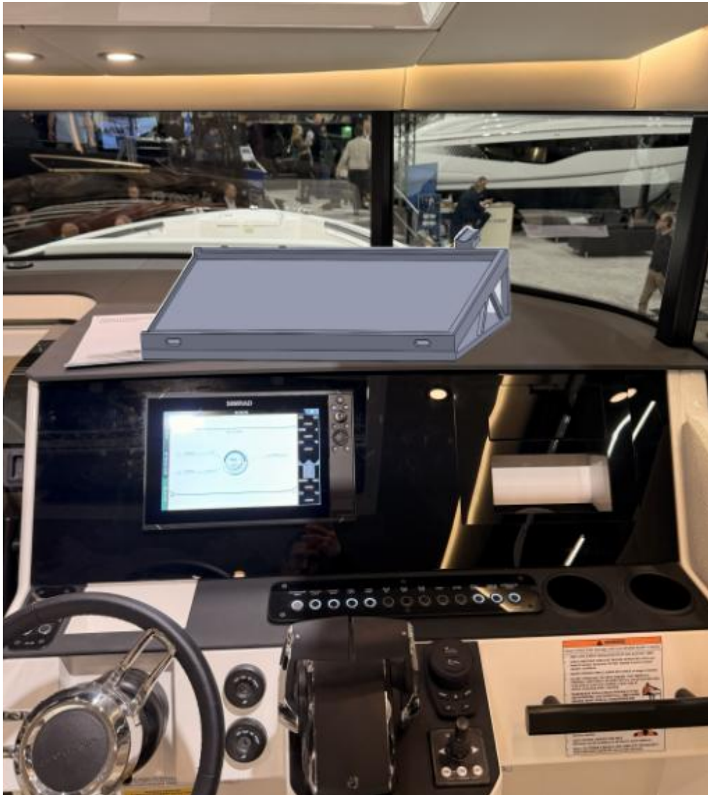
Figure 21. The nautical chart stand on a Saxdor 320 GTC, here for the operator of the vessel to use (Wilhelm Guarnieri, 2026)
