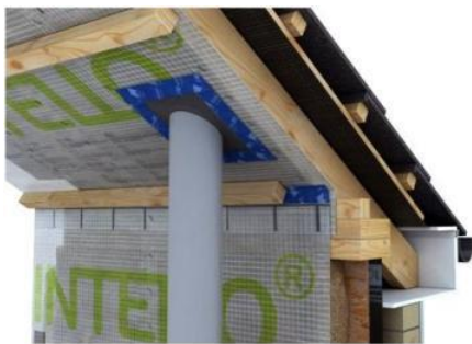
Figure 17. A Pro Clima brand service grummet sealing a pipe penetration of the airtightness layer [72].
