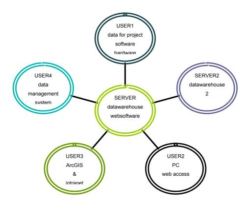
figure 28: Structure of a distributed GIS
