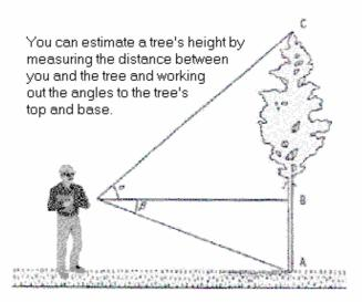
figure 43: Height measurement based on trigonometric principles (angles)
