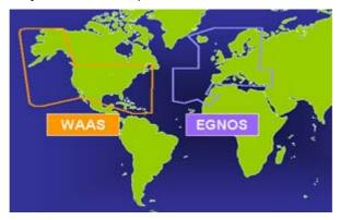
You can compare this system with the differential GPS system, but here the corrections of the ground stations are first sent to the geostationary satellites, which send the corrected information to the user on earth. Each receiver which supports WAAS/EGNOS can make use of these corrections. Accuracy with WAAS/EGNOS is less than 3 meters.
