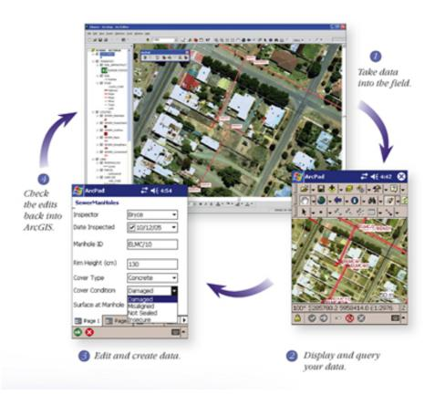
figure 2: Schematic view of the main use of ArcPad - ArcGIS
