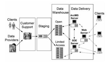
figure 34: structure of an EGIS, based on ESRI-software<sup>8</sup>
