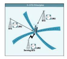
figure 30: Positioning by mobile antennas<sup>5</sup>
