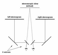
figure 40: Schematic view of a stereoscope
