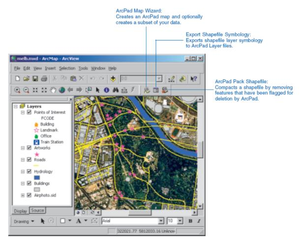
figure 65: ArcPad Tools for ArcGIS (source ArcPad Manual)
