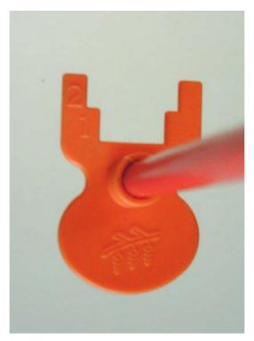
figure 100: Detail of the slot of the relascope
