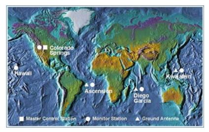
figure 12: Position of the Monitor Stations
