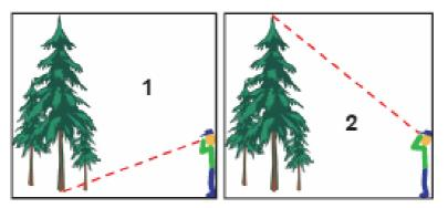
figure 104: Pointing towards birch point & top of the tree
