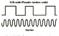
The trick is to find one particular carrier cycle and use it for timing.
