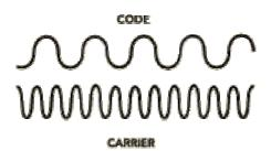
figure 19: Code frequency vs. Carrier frequency
