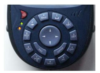
figure 8: Built-in alphanumeric keypad with backlight
