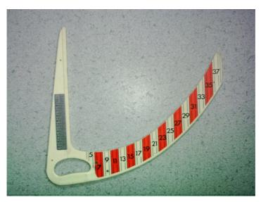
figure 41: Example of a tree calliper
