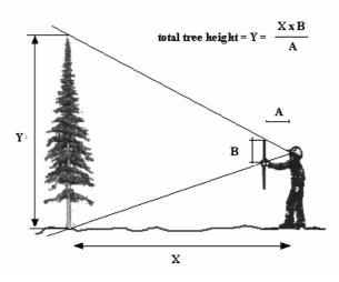
figure 42: Height measurement based on geometric principles (similar triangles)
