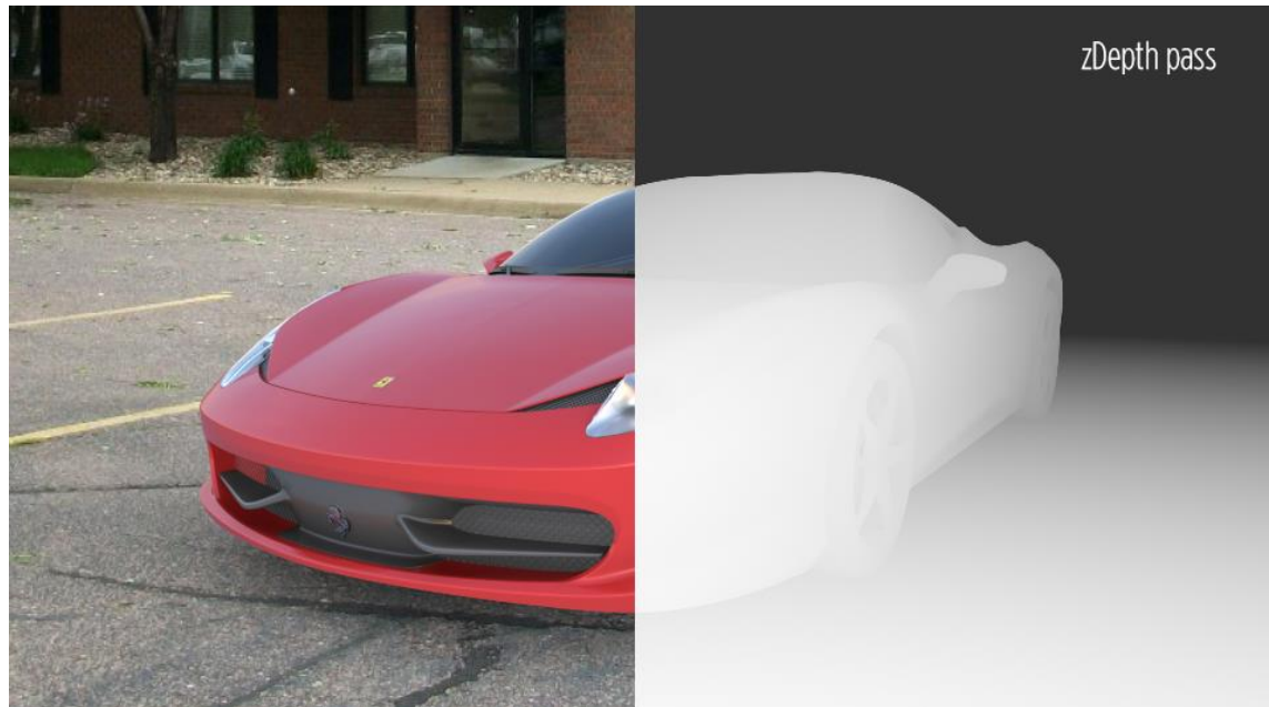
FIGURE 48. zDepth pass demonstration. The further away elements are from the camera, the darker are pixels in zDepth pass (Ostasheva, A. 2015)
