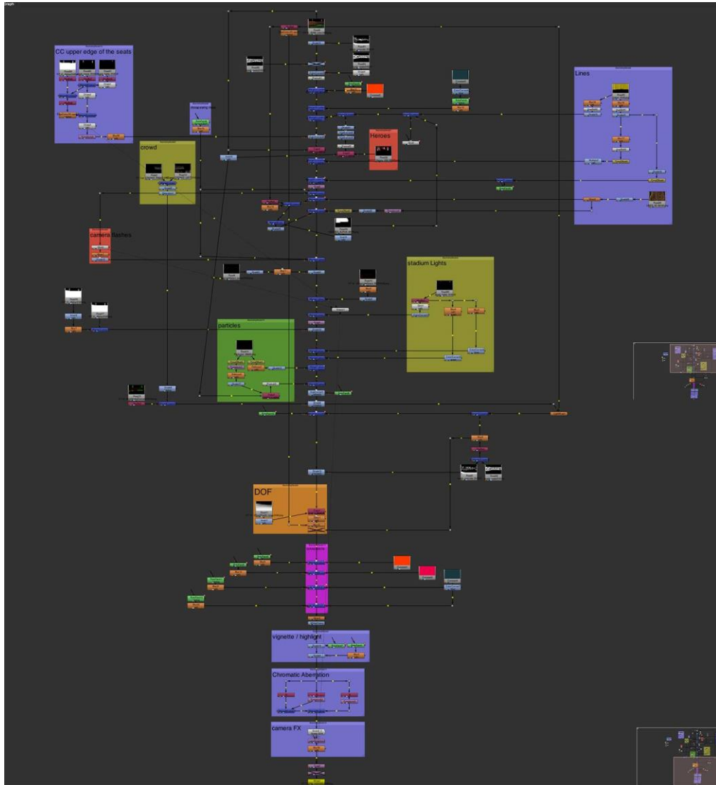
FIGURE 10. An example of a real-life node tree inside of NUKE.
