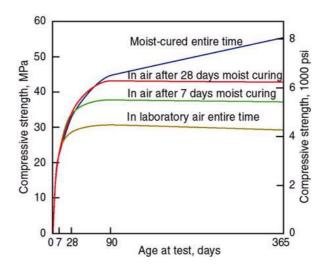
Figure 1. Moist curing time and compressive strength gain
