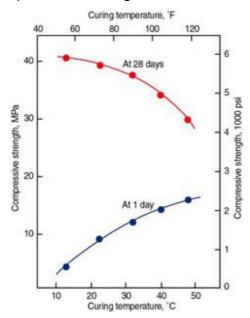
Figure 2. Effect of curing temperature on compressive strength
