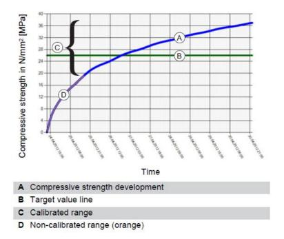
Figure 7. Compressive strength graph
