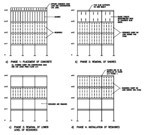
Figure 11. Typical construction phases
