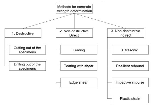
Figure 3. Classification of the methods to determine concrete strength
