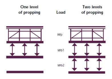
Figure 10. Diagrammatic presentation of reshoring
