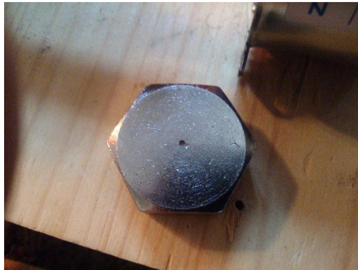
Figure 11. Die with 1.5 mm hole
